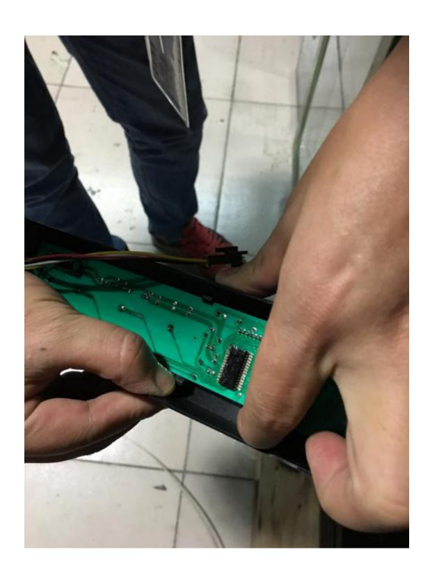
4. Replace with a new control board, install it in the holder.
