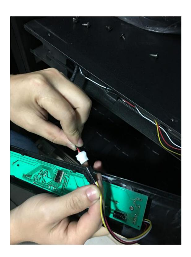
3. Unscrew the control board, Press and pull off the control board from the holder
