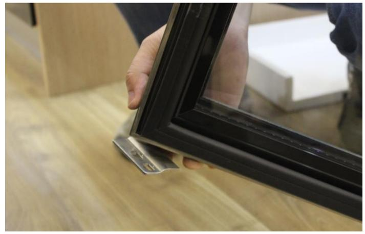
4. Fix the door and hinge on the unit body, the lower hinge should put against the two holes on the right of bottom grill and twist them.
