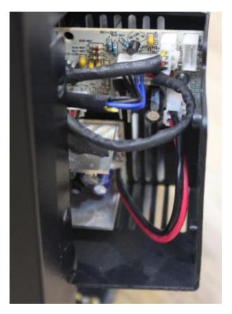
3. Disconnect the wirings by press and pull off the connectors. All 4 of the connectors are
