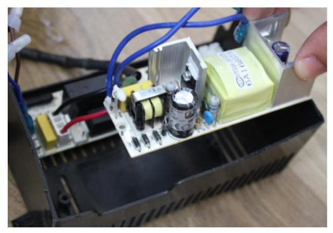
6. Replace with a new power board and fix it with screws.
