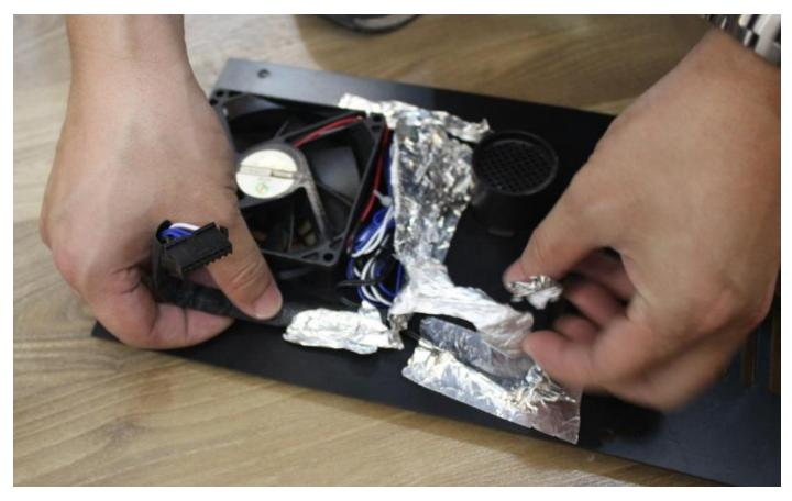
5. Cut off the strap and disconnect the wirings.
